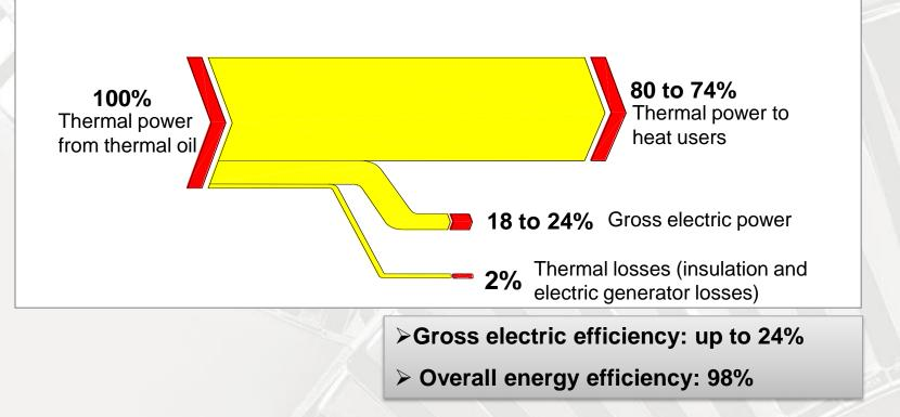
To better exploit the heat source (renewable or not) cogeneration should be strongly preferred as a way to utilize most of fuel/source energy content. *Note: Net efficiency from biomass shall take into account a furnace/boiler efficiency of about 83-88%*
