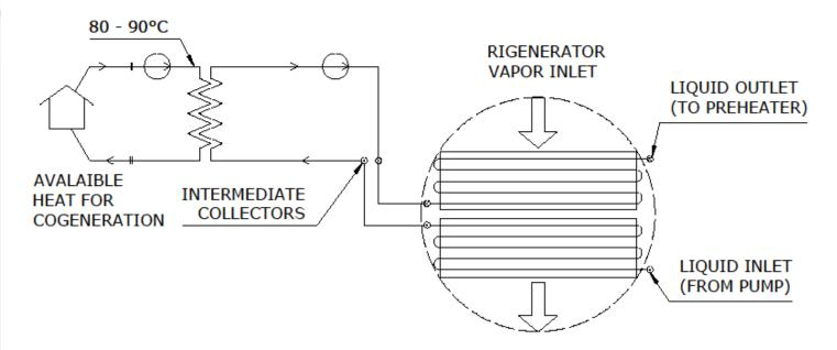
$\Rightarrow$ The additional circuit allows to utilize a fraction of the heat available in the regenerator to heat up a flow of water at a temperature higher than condenser temperature
