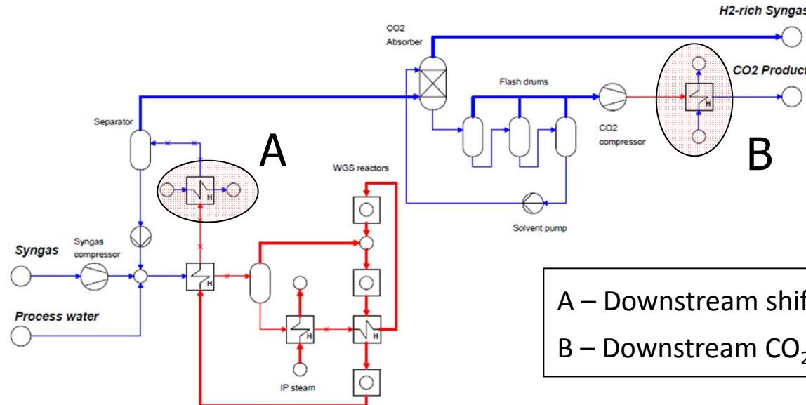
A – Downstream shifting section (137 °C/ 40 °C)
