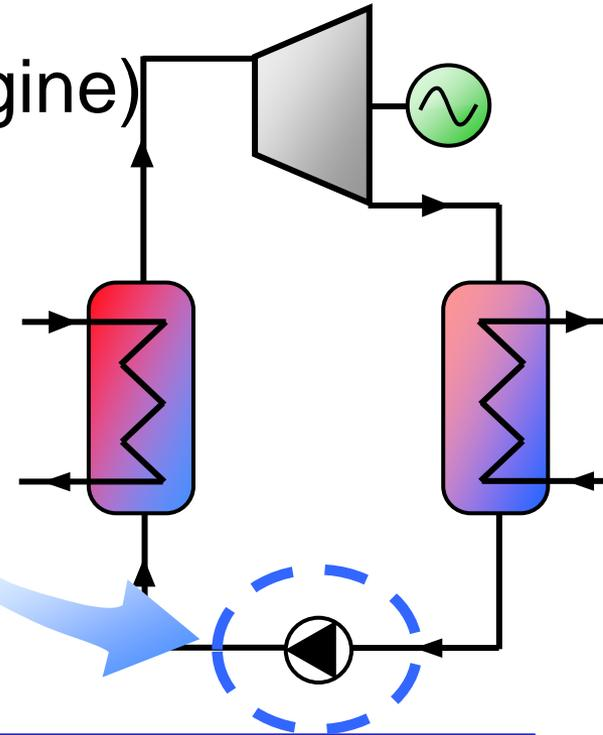
Downgrade ORC to “Pumpless” cycle for exploring cost-effective alternative
