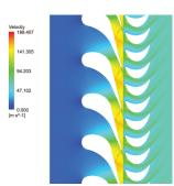
For the impulse turbine operating with R227ea fluid the supersonic nozzle was redesigned and proper outflow angle and degree of divergence were set. The velocity field is more uniform and as a result the internal efficiency of the stage rised by 3%.
