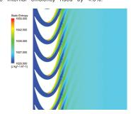
For the Curtis turbine operating with R227ea fluid the rotor profile was redesigned according to the flow kinematics. Significant reduction of the entropy in the rotor can beobserved. The internal efficiency benefit is 3%.
