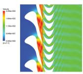
For the impulse turbine operating with HFE7100 fluid the rotor profile was redesigned according to the flow kinematics. The separation of the flow was significantly reducedand thus the internal efficiency rised by 4.5%.
