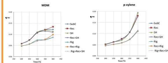
PERFORMANCE INDEX @ optimum design point for different fluids and different ORC configurations
