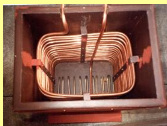
Fig. 1. View of evaporator
